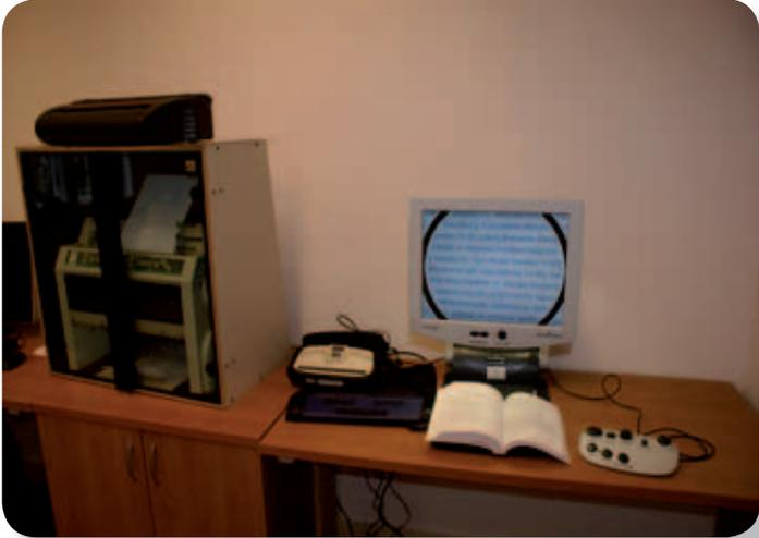
Image 1. A Braille printer, a Braille SENSE notetaker and an enlarger
